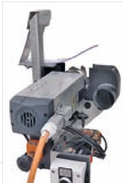
The Grooving Unit creates grooves and performs milling operations on the underside of the panel.
