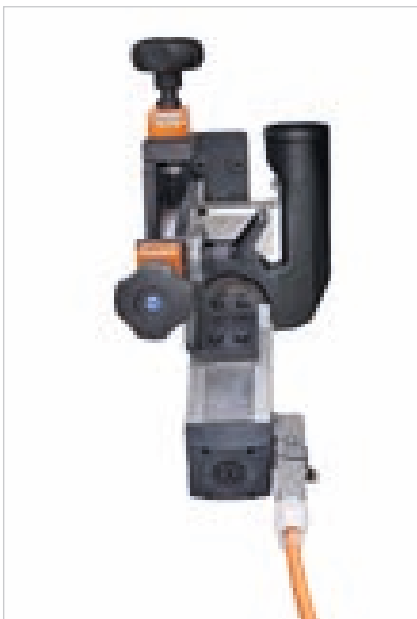
The Rough Trimmer reduces the excess edge on the upper part of the panel.
