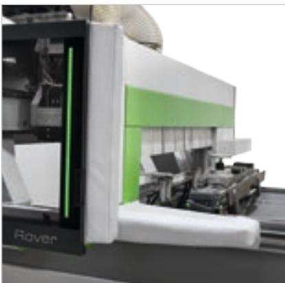
Safety and flexibility thanks to the new bumpers combined with photocells with no footprint and dynamic tandem loading.
