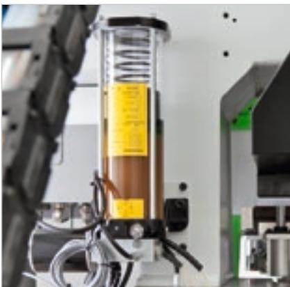
**Automated lubrication** ensures the continuous lubrication of the machine's main moving parts without the need for operator intervention.
