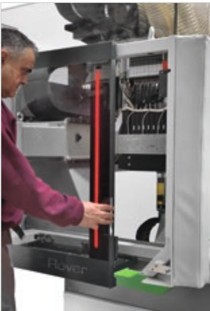
**Facilitated access** during tool change operations thanks to the openable front hood.
