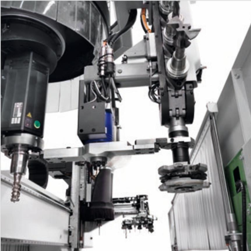
**Independent Y axis** allows tool changes whilst the machine is running, using the largest possible number of tools available in the magazine. The **shuttle** in the vertical chain magazine speeds up the tool change operation.
