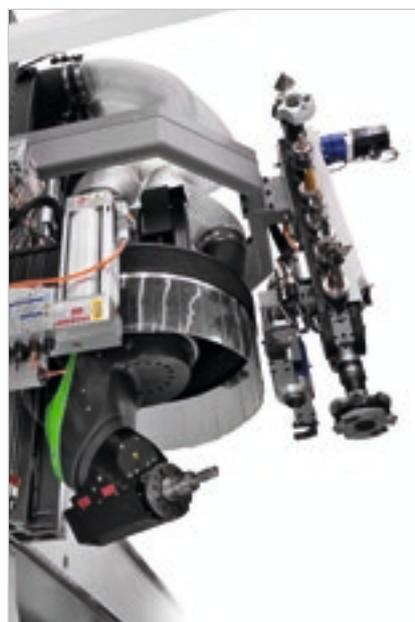
**Vertical chain tool magazine** on Y axis with 10-15 positions.
