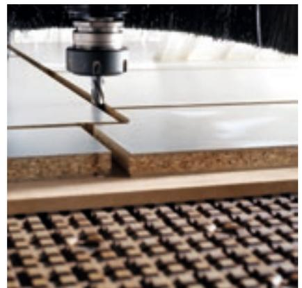
Two machines in one: the full functionality and quality of a true pantograph table is guaranteed by the **CFT (Convertible Flat Table)**, which supports the machining of thin panels, nesting and folding on a machine equipped with a roller bar table.
