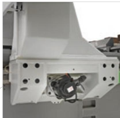
The **double X-axis motorisation** supports high speeds and accelerations whilst ensuring high quality finish and precision.
