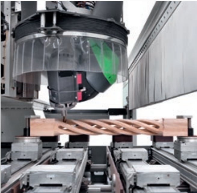
↙ 5-axis milling unit with 360mm hood with adjustable height.
