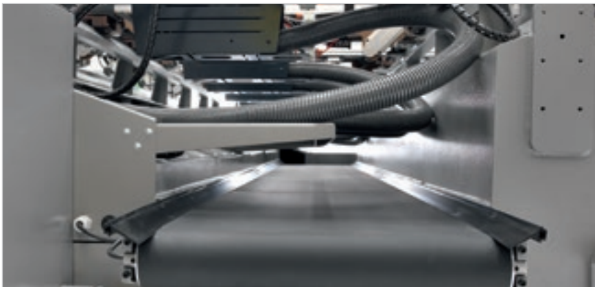
Motorised conveyor belt for the removal of chips and waste.
