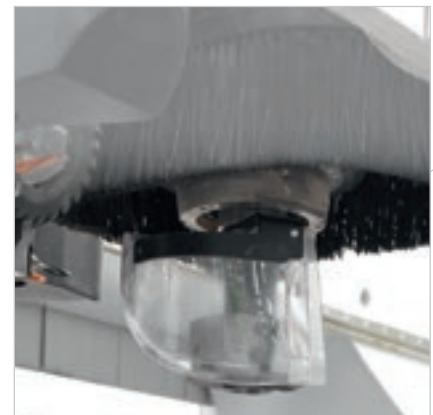
Integrated deflector (chip conveyor) managed via the NC.
