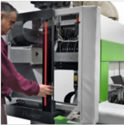
New hood with openable Lexan front door, for ease of operation.
